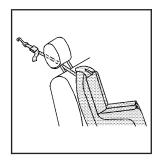
If the position you are using has an adjustable head restraint and you are using a single tether, route the tether under the head restraint and in between the head restraint posts. See *Head Restraints on page 15*.
